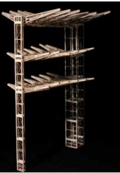
1:100 Model of the primary structure of the facility
